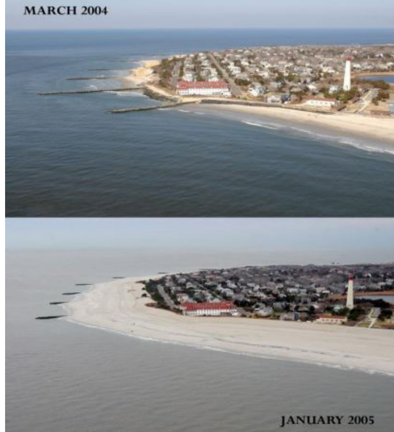
Beach replenishment on the state park beach and around Cape May Point, before (top) and after (below) the restoration. Source: U.S. Army Corps of Engineers 2007.
